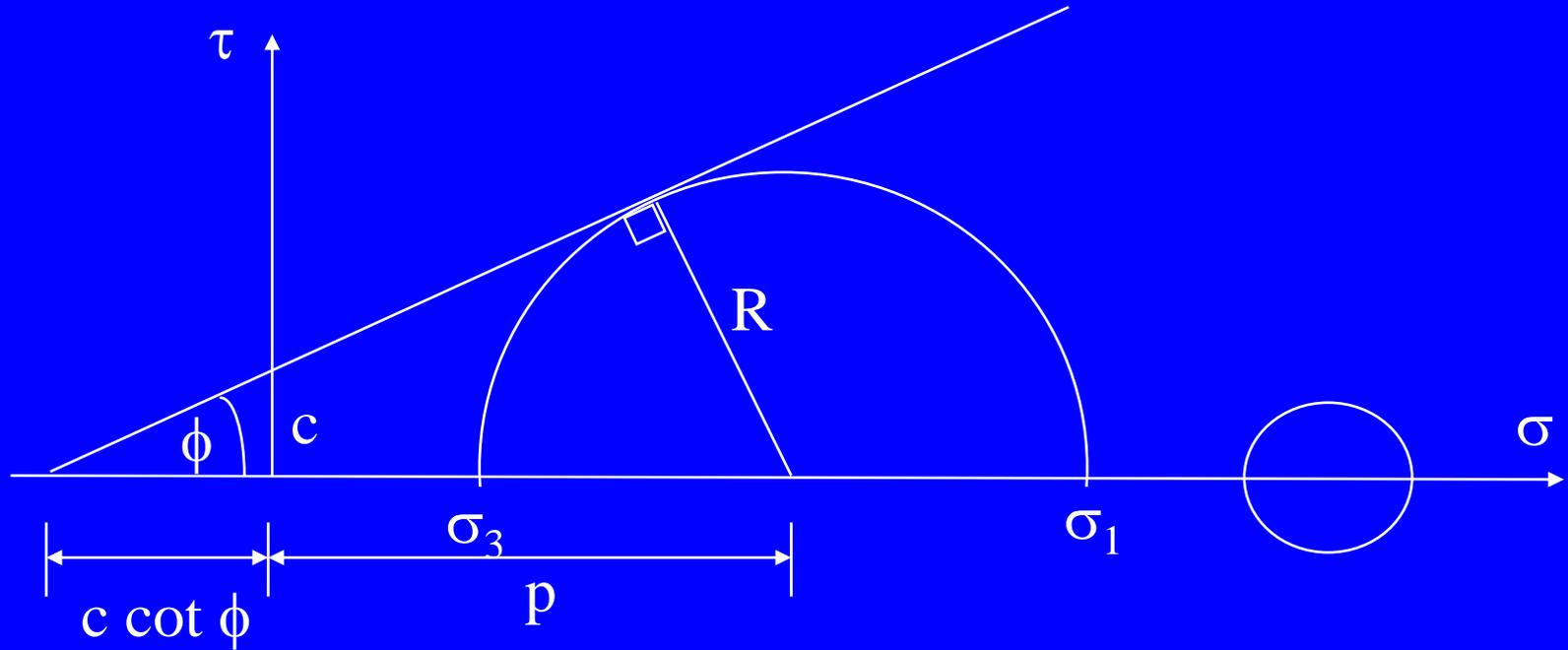
Failure occurs if a Mohr circle touches the failure criterion. Then
