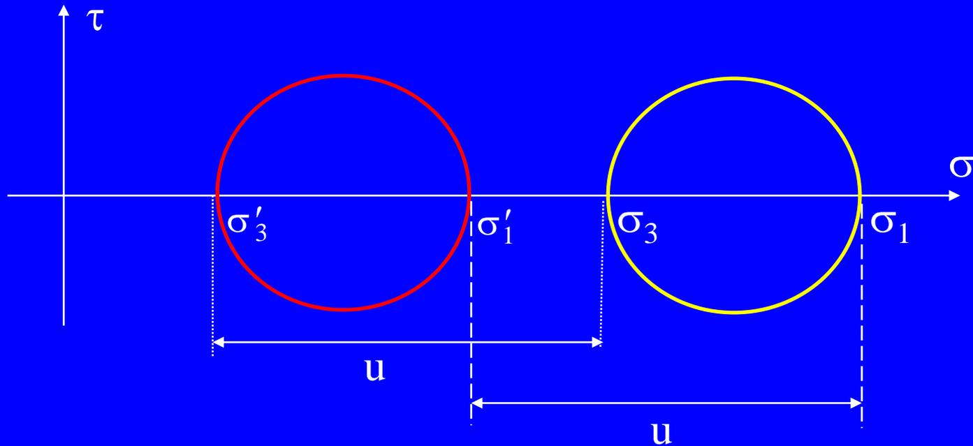
For any point in the soil a total and an effective stress Mohr circle can be drawn. These are the same size with
