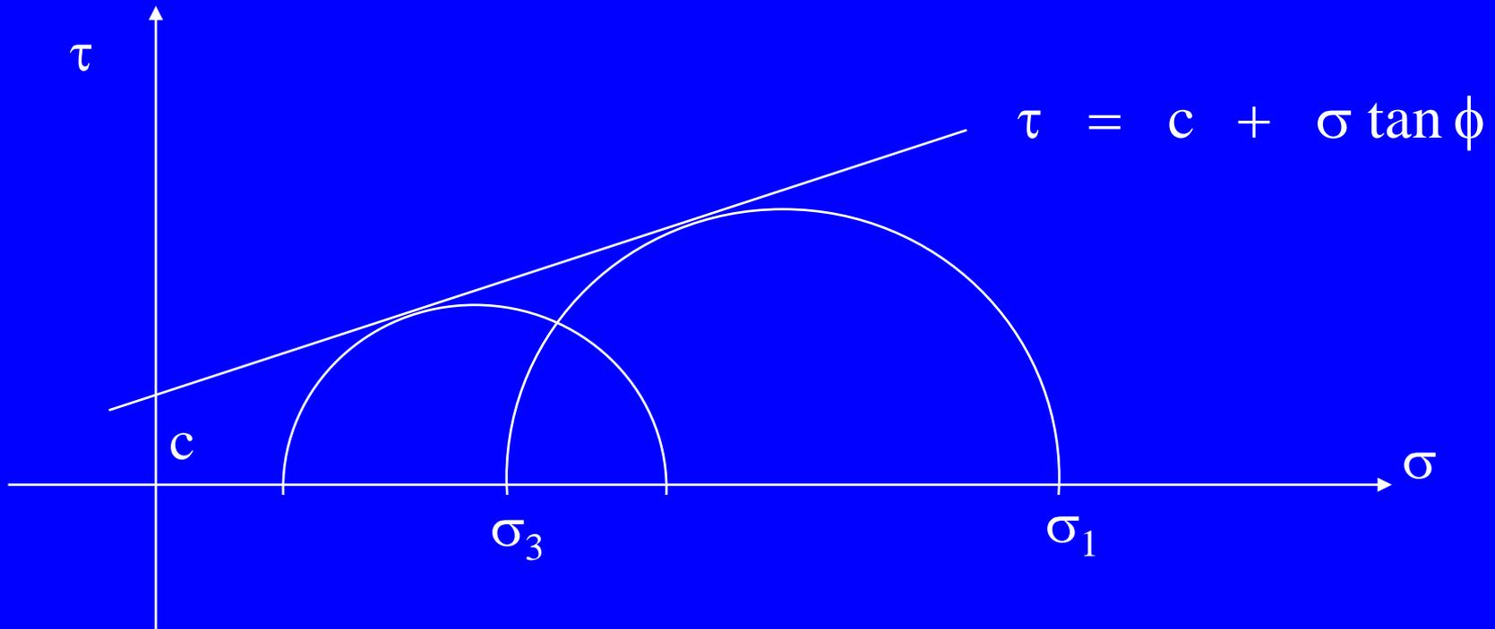
The Mohr-Coulomb failure locus is tangent to the Mohr circles at failure
