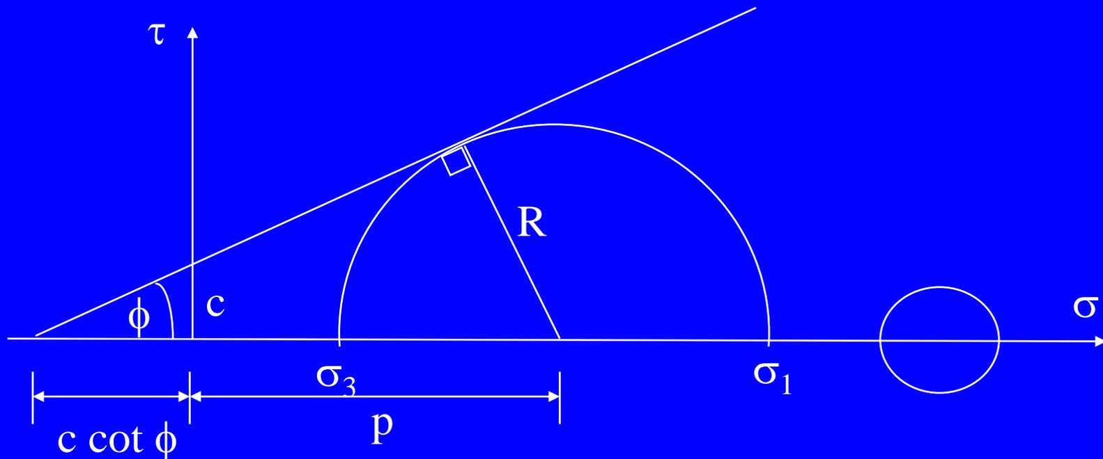
Failure occurs if a Mohr circle touches the failure criterion. Then
